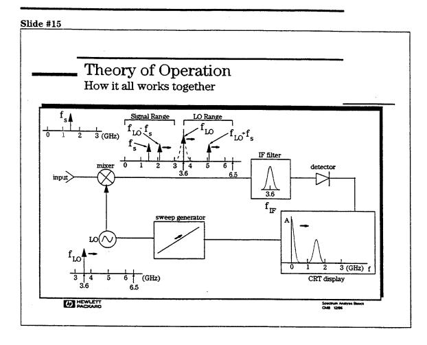
Let's see how these components work together to make a spectrum analyzer. Note that while the RF input attenuator, IF gain, and video filter are important components, they are not critical when describing how the analyzer works.
