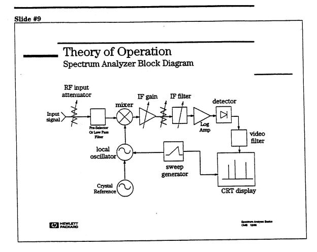
The major components in a spectrum analyzer are the RF input attenuator, mixer, IF (Intermediate Frequency) gain, IF filter, detector, video filter, local oscillator, sweep generator, and CRT display. Before we talk about how these pieces work together, let's get a fundamental understanding of each component individually.
