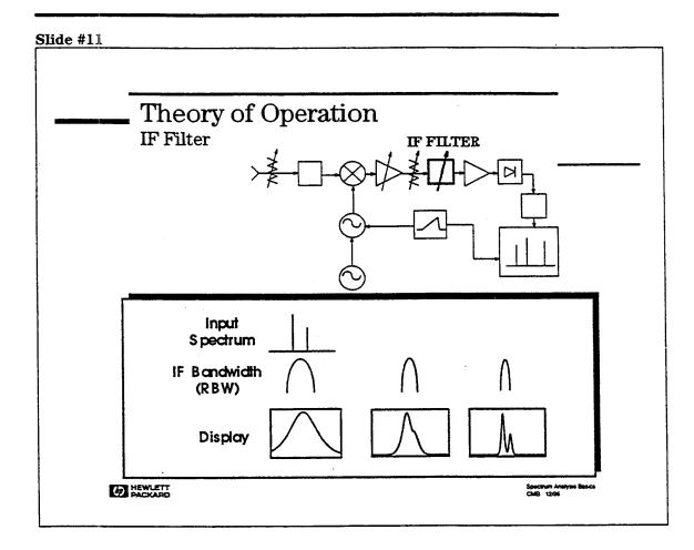
The IF filter is a bandpass filter which is used as the "window" for detecting signals. It's bandwidth is also called the resolution bandwidth (RBW) of the analyzer and can be changed via the front panel of the analyzer.
